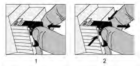
Figure 5: Installing / removing the protective cap
