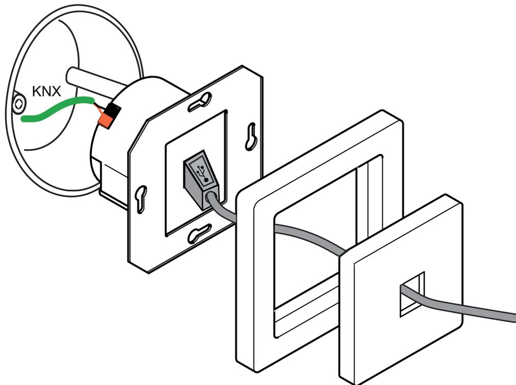
Figure 4: Device connection (FM design)
